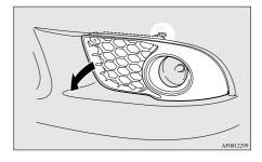
3. Remove the screws (B) and pull the entire lamp unit out.
