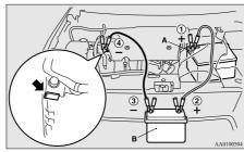
7. Connect one end of the other jumper cable to the negative (-) terminal of the booster battery, and the other end to the engine block of the vehicle with the discharged battery at the point farthest from the battery.
