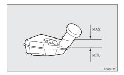
The fluid level is monitored by a float. When the brake fluid level falls below the "MIN" mark, the brake fluid warning lamp lights up.
