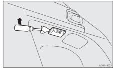
2. Remove the bulb by pulling it out.
