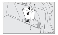
Check to make certain that the AWC control fluid level is always between the "MAX" and "MIN" level markings on the fluid reservoir and top up the fluid, if necessary.
