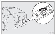
2. Remove the bulb by pulling it out.
