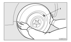
7. Finger-tighten the wheel nuts.
