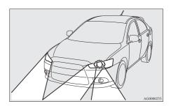
When the steering wheel is turned (on a curve, for example), the road ahead in the direction in which the vehicle is being turned is illuminated. (The left bending lamp comes on when the vehicle is turned leftward, and the right bending lamp comes on when the car is turned rightward.)
