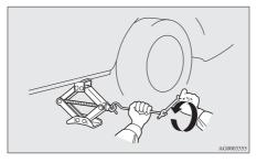
Tighten the nuts in the order shown in the illustration until each nut has been tightened to the torque listed here.
