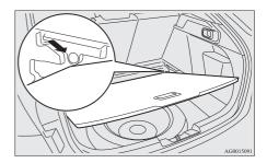
3. Push the board in all the way with the front part lowered, and lower the board.
