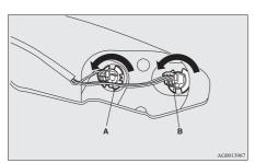
A- Rear turn-signal lamp B- Stop and tail lamp
