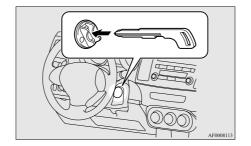
8. Insert the keyless operation key into the emergency key.
