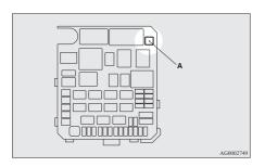
4. Insert a new fuse of the same capacity by using the fuse puller and insert the fuse at the same place in the fuse block.
