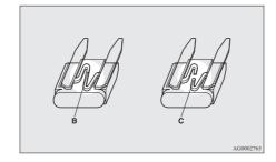
B- Fuse is OK C- Blown fuse
