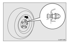
• If all 4 aluminium wheels are changed to steel wheels, e.g. when fitting winter tyres, use tapered nuts.
