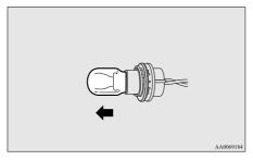
3. To install the bulb, perform the removal steps in reverse.
