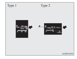
The "\(\vec{\pi}\)" mark (A) in the momentary fuel gauge shows the average fuel consumption.
