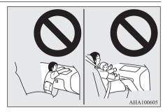
Use rearward facing child restraints in the rear seat or turn off the front passenger's airbag ON-OFF switch (if so equipped). (Refer to "To turn an airbag off" on page 4-28)
