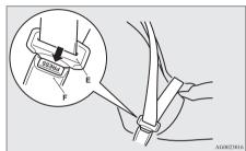
2. Push the button (G) on the buckle (C) using the latch plate (E) to disconnect the seat belt from the buckle.
