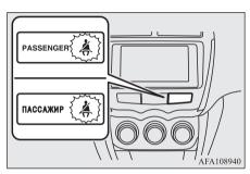
The lamp comes on when a person sits on the front passenger seat but does not fasten the seat belt. It goes off when the seat belt is subsequently fastened.
