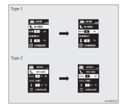
3. Press and hold the multi-information meter switch for about 2 seconds or more to switch in sequence from A or 1 (Auto reset mode) → M, 2 or P (Manual reset mode) → A or 1 (Auto reset mode).
