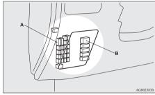
A- Main fuse block B- Sub fuse block 1. Insert a straight blade (or minus) screwdriver into the notch of the fuse lid and pry gently to remove it.
