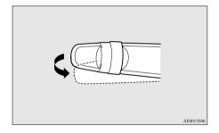
4. The headlamps will come on in the lowbeam setting for about 30 seconds. After the headlamps go off, the headlamps can be turned on again in the low beam setting for about 30 seconds by pulling the turn signal lever towards you within 60 seconds of turning the ignition switch to the "OFF" position or putting the operation mode in OFF
