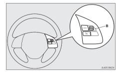
To slow down your speed in small amounts, push down the SET - switch for less than about 1 second and release it.
