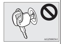
In cases like these, remove the object or additional key from the vehicle key. Then try again to start the engine. If the engine does not start, we recommend you to con-
