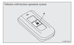
The settings mode can be toggled by pressing the UNLOCK switch. The mode can be confirmed from the number of times the buzzer sounds.
