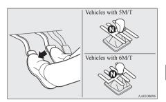
Release the clutch pedal. The "sssd" display/indicator will turn on and the engine will stop automatically.
