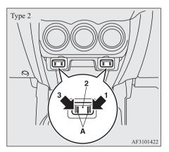
1 (HI) - Heater high (for quick heating).
