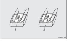
B- Fuse is OK C- Blown fuse
