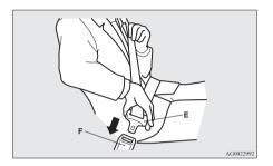
Make sure the lap belt is positioned as low as possible on the hips and pull the shoulder belt to adjust the slackness of the lap belt.
