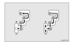
While depressing the brake pedal, move the selector lever through the gate.
