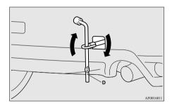
4. Always attach the tow rope to the towing hook. Otherwise, the instructions are the same as for "When being towed by another vehicle". When finished towing, remove the towing hook, and stow it in the specified location.
