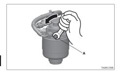
Pump the hand pump (B) until there are no more bubbles in the fuel coming out of the air plug (A). When doing this, place a cloth around the air plug (A) to prevent the escaping fuel from spraying out.
