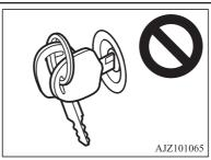
In cases like these, remove the object or additional key from the vehicle key and turn the key back to the "ACC" or "LOCK" position. Then try again to start the engine. If the engine does not start, we recommend you to contact your MITSUBISHI MOTORS Authorized Service Point.
