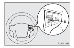
If the current vehicle speed is lower than about 30 km/h (19 mph) (settable minimum speed), the set speed is set at about 30 km/h (19 mph).
