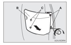
3. Turn the socket anticlockwise and remove it, and then pull the bulb out of the socket.
