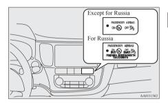
The both indicator normally comes on when the operation mode of the power switch is put in ON, and goes off a few seconds later.
