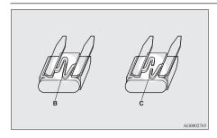
B- Fuse is OK C- Blown fuse
