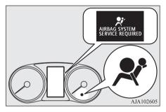
There is a Supplemental Restraint System ("SRS") warning lamp on the instrument panel. The system checks itself every time the operation mode of the power switch is put in ON. The SRS warning lamp will come on for several seconds and then go out. This is normal and means the system is working properly.
