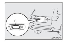
If the open switch is pressed with the tailgate and all doors are unlocked, the electric tailgate opens after the warning buzzer sounds and the hazard warning flasher blinks.
