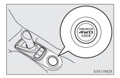
When the 4WD LOCK mode is activated, the above display appears on the information screen in the multi-information display for some seconds.
