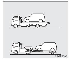
In the following cases, contact a MITSUBISHI MOTORS Authorized Service Point and transport the vehicle with all wheels on a carriage.
