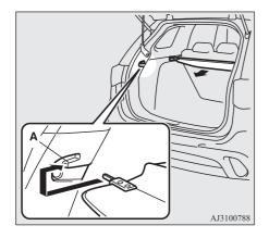
Remove the cover from the mounting grooves, and the cover will roll back into the retracted position.
