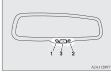
When the operation mode of the power switch is put in ON, the green indicator (1) illuminates and the reflection factor of the mirror is automatically changed.
