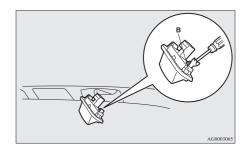
3. Remove the bulb from the socket.
