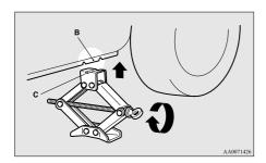
4. Check that the flange portion at the jacking point fits in the groove at the top of the jack.
