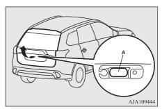
The tailgate cannot be opened when the battery is flat or disconnected.
