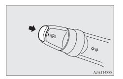
The automatic high-beam system is activated and the indicator will illuminate. If the automatic high-beam system switch is pressed again, the automatic high-beam system will be deactivated and the automatic high-beam system indicator will go off.
