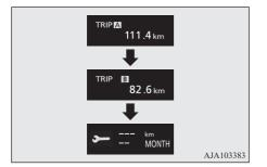
2. Press and hold the multi information display switch for about 2 seconds or more to display ">=" and make it flash. (If there is no operation for about 10 seconds with flashing, the display returns to the previous screen.)
