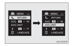
Press and hold the multi information display switch for about 2 seconds or more to display "AVG UNIT".
