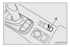
When the brake auto hold system cannot be used, a buzzer will sound and the message will appear on the information screen in the multi information display.
