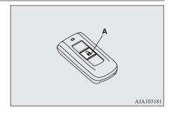
The settings mode can be toggled by pressing the UNLOCK switch. The mode can be confirmed from the number of times the buzzer sounds.
