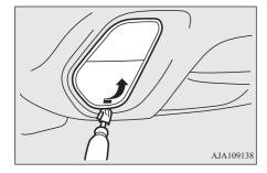
2. Turn the socket (A) anticlockwise to remove it, and then pull the bulb out of the socket.
