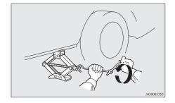
9. Tighten the nuts in the order shown in the illustration until each nut has been tightened to the torque listed here.
