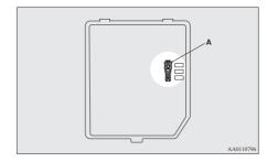
3. Referring to the fuse load capacity table, check the fuse pertaining to the problem.
