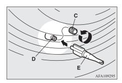
7. Remove the valve insert (F) by turning it anticlockwise using the valve remover (E). Put the removed valve insert in a clean place so it does not get dirty.
