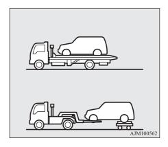
In the following cases, contact a MITSUBISHI MOTORS Authorized Service Point and transport the vehicle with all wheels on a carriage.
