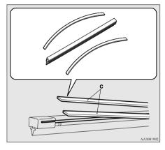
Insert the wiper blade into the arm, starting with the opposite end of the blade from the stopper. Make sure the hook
