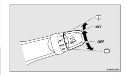
The wiper operates continuously for several seconds then operates intermittently at intervals of
