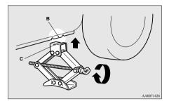
Check that the flange portion at the jacking point fits in the groove at the top of the jack.
