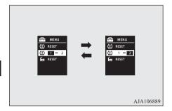
The valid tyre ID set is changed, and the number of the tyre pressure monitoring system (TPMS) SET indicator is changed.
