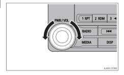
Turn the PWR/VOL key clockwise to increase, and counter- clockwise to decrease the volume.
