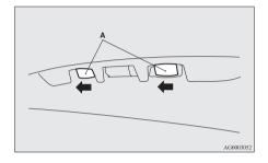
Insert a minus screwdriver with the end covered with a cloth or other object to press the hook (B) aside and remove the lens.
