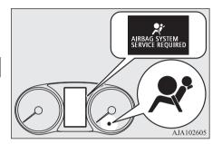
There is a Supplemental Restraint System ("SRS") warning lamp on the instrument panel. The system checks itself every time the operation mode of the power switch is put in ON. The SRS warning lamp will come on for several seconds and then go out. This is normal and means the system is working properly.
