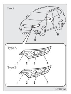
Type A: Halogen headlamps type Type B: LED headlamps type
