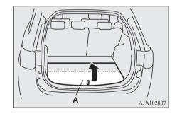
To use the luggage floor box in the rear seat side, insert your hand in the gap (B) and raise the board (A) to the seat side.
