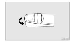
4. The headlamps will come on in the low beam setting for about 30 seconds. After the headlamps go off, the headlamps can be turned on again in the low beam setting for about 30 seconds by pulling the turn signal lever towards you within 60 seconds of putting the operation mode in OFF.
