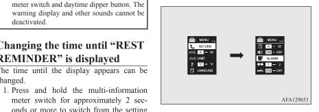
3. Press and hold the multi-information meter switch for approximately 2 seconds or more to display "ALARM" (rest time setting).
