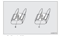
B- Fuse is OK C- Blown fuse
