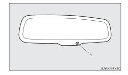
When the ignition switch is turned to the "ON" position or the operation mode is put in ON, the reflection factor of the mirror is automatically changed.
