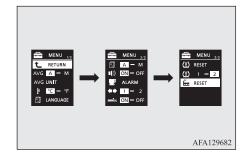
3. When you press and hold the multi-information meter switch for approximately 5 seconds or more, the buzzer sounds and all of the function settings are returned to the factory settings.
