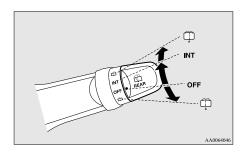
INT- The wiper operates continuously for several seconds then operates intermittently at intervals of about every 8 seconds
