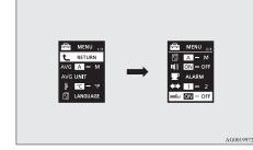
3. Press and hold the multi-information meter switch for approximately 2 seconds or more to switch in sequence from ON (with the green bar graph) → OFF (without the green bar graph) → ON (with the green bar graph).
