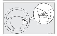
A- CRUISE CONTROL ON/OFF switch Used to turn on and off the cruise control.
