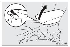
The tissue holder and pen holder are located on the underside of the floor console box lid.
