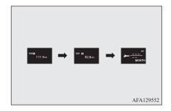
2. Press and hold the multi-information meter switch for approximately 2 seconds or more to display ">=" and make it flash. (If there is no operation for approximately 10 seconds with flashing, the display returns to the previous screen.)
