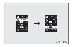
Press and hold the multi-information meter switch for approximately 2 seconds or more to switch in sequence from °C → °F → °C.
