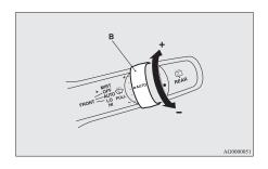
"+"- Higher sensitivity to rain "-"- Lower sensitivity to rain
