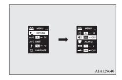
3. Press and hold the multi-information meter switch for approximately 2 seconds or more to switch in sequence from ON (operation sound on) → OFF (operation sound off) → ON (operation sound on).
