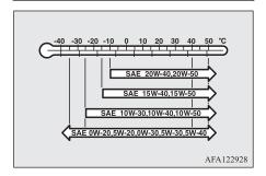
Use engine oil conforming to the following classification:
