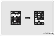
3. Press and hold the multi-information meter switch for approximately 2 seconds or more to switch in sequence from 1 (turn-signal sound 1) → (turn-signal sound 2) → 1 (turn-signal sound 1). The setting changes to the selected turn-signal sound.
