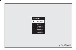
Press and hold the multi-information meter switch for approximately 2 seconds or more to change the setting to the selected unit.
