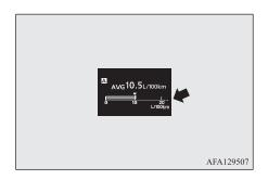
When the value of momentary fuel consumption surpasses the value of average fuel consumption, the momentary fuel consumption is displayed with a white bar graph.
