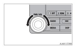
Turn the PWR/VOL key clockwise to increase, and counter- clockwise to decrease the volume.
