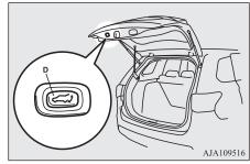
If the close switch on the inside of the electric tailgate is pressed, the electric tailgate closes after the warning buzzer sounds.
