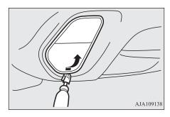
2. Turn the socket (A) anticlockwise to remove it, and then pull the bulb out of the socket.
