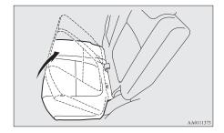
5. Flip the seat cushion forward. On vehicles with the third seats, move the lever (A) to the luggage area mode position.
