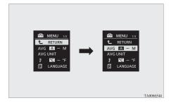
3. Press and hold the multi information display switch for about 2 seconds or more to switch from A/1 (Auto reset mode) to M/2/P (Manual reset mode), or from M/2/P to A/1.
