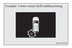
Even after the buzzer and display has stopped warning, the indication lamp (A) on "SONAR" switch will continue blinking until the system reverts to the normal state. Have the vehicle inspected at a MITSUBISHI MOTORS Authorized Service Point.
