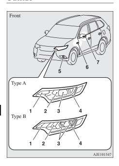
Type A: Halogen headlamps type Type B: LED headlamps type
