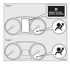
There is a Supplemental Restraint System ("SRS") warning lamp on the instrument panel. The system checks itself every time the ignition switch is turned to the "ON" position or the operation mode is put in ON. The SRS warning lamp will come on for several seconds and then go out. This is normal and means the system is working properly.
