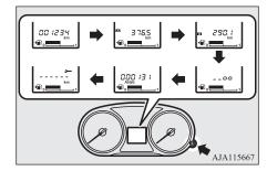
2. Press and hold the multi information display switch for about 2 seconds or more to make the spanner mark start flashing. (If there is no operation for about 10 seconds with flashing, the display will revert to its original indication.)
