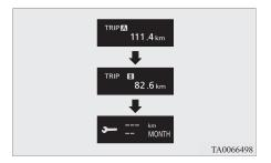
2. Press and hold the multi information display switch for about 2 seconds or more to display ">=" and make it flash. (If there is no operation for about 10 seconds with flashing, the display returns to the previous screen.)
