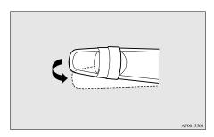
4. The headlamps will come on in the low beam setting for about 30 seconds. After the headlamps go off, the headlamps can be turned on again in the low beam setting for about 30 seconds by pulling the turn signal lever towards you within 60 seconds of turning the ignition switch to the "LOCK" position or putting the operation mode in OFF.
