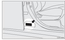
The label shows model code, engine model, transmission model and body colour code, etc.
