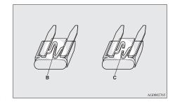
B- Fuse is OK C- Blown fuse
