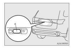
If the open switch is pressed with the tailgate and all doors are unlocked, the electric tailgate opens after the warning buzzer sounds. When the tailgate and all doors are locked, the warning buzzer will not sound.
