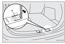
2. Loosen the tyre hanger installation bolt by turning it anticlockwise with the wheel nut wrench.
