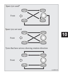
\*: If the spare tyre wheel differs from the standard tyre wheel, do not perform tyre rotation using a spare wheel.
