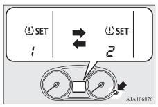
3. The valid tyre ID set is changed, and the number of the tyre pressure monitoring system (TPMS) SET indicator is changed.
