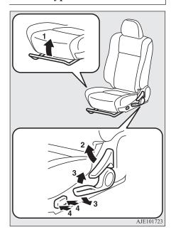
1- To adjust forward or backward Lift the handle and adjust the seat to the desired position, and release the handle. Т.
