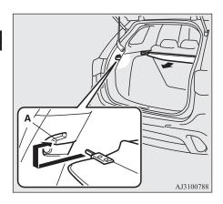
2. Remove the cover from the mounting grooves, and the cover will roll back into the retracted position.
